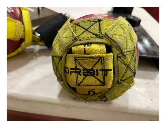
Can you provide any other view of this weight? The reason I ask is that it appears that the added bottom portion is a patch. By rule, the structural straps are not sewn together and do not form an X under the head of the weight. I would like another view because, from this picture, the implement looks to be illegal.
